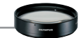
Underwater Macro Conversion Lens PTMC-01 Underwater approx. 2X (area ratio) • Lens construction: 2 elements in 1 group • Size: φ70 mm x 18 mm Weight: 146 g • Lens mount diameter: φ67 mm • The tip is provided with a 67 mm diameter filter thread for stacking with other lens filter or lens.
