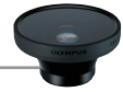
Underwater Wide Conversion Lens PTWC-01 Underwater approx. 0.6X (underwater angle of view approx. 100°) • Lens construction: 4 elements in 4 groups • Size: φ131 mm x 69 mm Weight: 1,000 g • Lens mount diameter: φ67 mm • When used on land, the four corners of the image get cropped.
